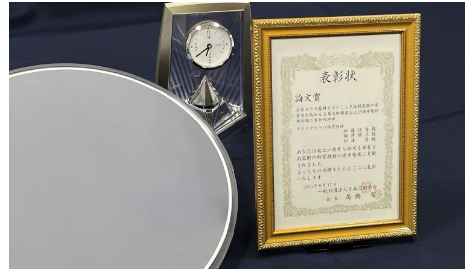
Left side of photo: Quartz glass component coated with ceramic thermal spray coating
